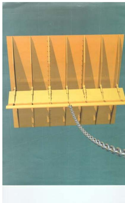
Figure B-6 Illustration of the BLADE anchor.
